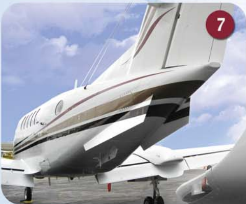
Installation of Raisbeck Dual Aft Body Strakes completed
