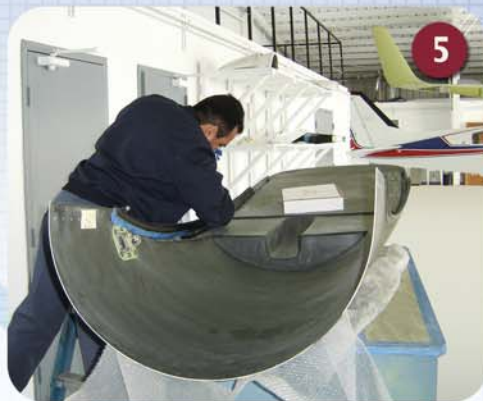
Preparing the wing locker for installation
