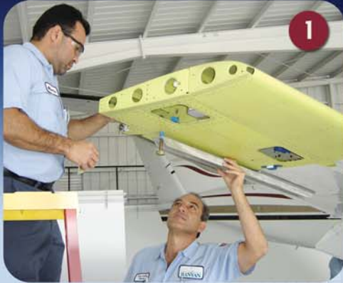
Banyan technicians install new wing extension
