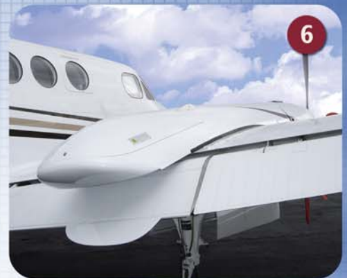
Installation of Nacelle Wing Locker complete
