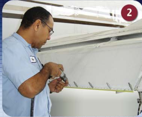
Installation of new gunney flap modification
